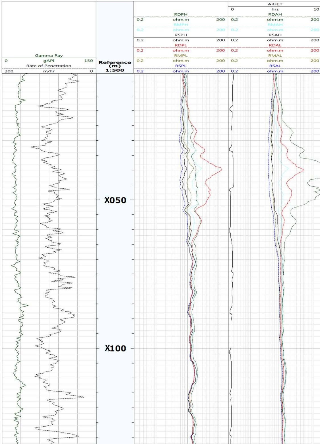
Hydrocarbon bearing formations in the reservoir can be identified with Resistivity tools, when Gamma readings are inadequate.
