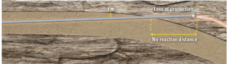
**At-the-bit measurement - Reactive steering**
