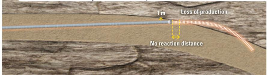
**PeriScope HD real-time boundary mapping - Proactive steering**
